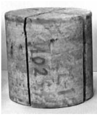
Fig. 6. Fracture directions on limestone specimens.
