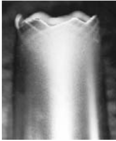
Fig. 5. Fracture directions in 12KhN3A steel specimens.
